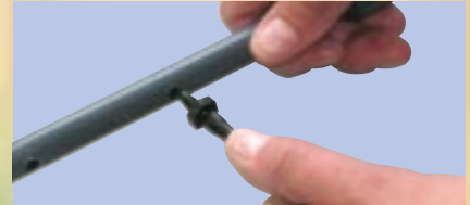
c. Attach complete lead to delivery tube by screwing threaded nipple into grey tube
